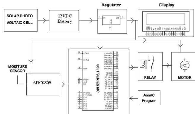
**Fig.2.1** Block Diagram Of Solar Power Irrigation
